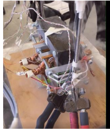
Fig. 8. The magnet test setup when the magnet had just been removed from the LN 2 bath but HTS currents continued to circulate for about 10 s.
