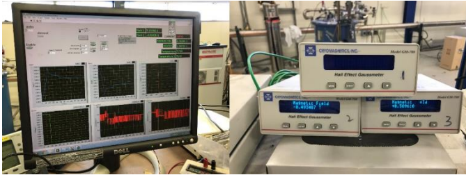
Fig. 10. The HTS magnet test monitoring system.
